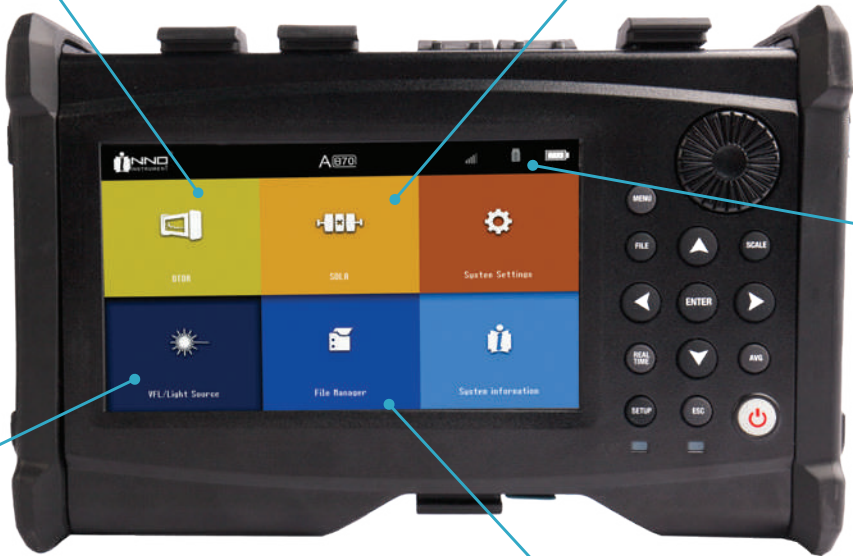
7" Touch Screen Smart GUI High Brightness Resolution of 800x480
